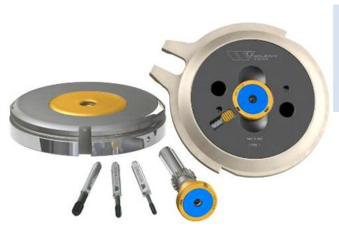
The Wilson Tapping Tool for Trumpf and Pullmax machines can be used to produce a thread in a punched or extruded hole in sheet metal. The Tapping Tool forms the thread rather than cutting, giving a stronger thread and not generating swarf.
