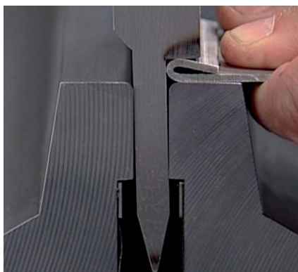
Pre-bend and flattening in the same tool.
