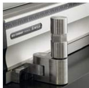
When using "HD" Tool Holders, it is possible to install 'pillars' to further support very wide and heavy bottom tools. These pillars offer additional stability to tools during the bending process. Available every 255 mm on front and backside.
