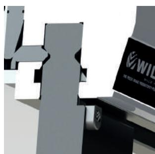
Tools are clamped using a pneumatically-controlled pair of self-adjusting wedges. When the wedges are engaged (clamped), they become an integral part of the tool.
