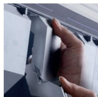
The Safety-Click® is WILA's patented safety mechanism which has been integrated into top tools with a weight up to 12,5 kg. This revolutionary mechanism allows tools to be changed vertically by simply clicking them in and out of the Clamping.
