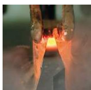
Almost all press brake tools produced by WILA are CNC-Deephardened®. The same applies to WILA's New Standard Premium Tool Holders. This makes them extremely robust and durable. Our New Standard Premium Tool Holders are hardened as shown here.
