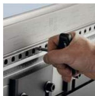
If bottom tool changeovers are not needed often, Premium and Pro Crowning/Bottom Tool Holder models with manual clamping are available as well. Manual Clamping is achieved via clamping bolts at a distance of every 25 mm, in the center 1000 mm and every 100 mm towards each end, allowing the clamping of tool segments as small as 15 mm in length.
