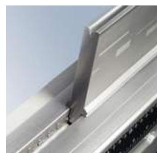
The V-Lock® improves the clamping and positioning of bottom tools. A groove in the tool tang allows specially designed clamping pins to automatically align and firmly clamp bottom tools in both X and Y directions.
