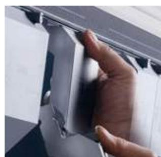
The Safety-Click® is WILA's patented safety mechanism which has been integrated into top tools with a weight up to 12,5 kg. This revolutionary mechanism allows tools to be changed vertically by simply clicking them in and out of the Clamping.
