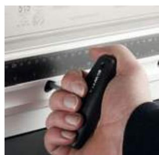
Ty-adjustment is crucial in achieving parallelism between top and bottom tools. Adjustment in Y direction makes it possible to fully compensate for unavoidable - cumulative - machining tolerances in the press brake. Either the top or bottom Tool Holder must be able to do this if one wants to achieve accurate and consistent bending results.
