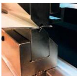
In addition to the range of top and bottom tools, WILA also offers a wide range of accessories. These include special inserts for making offset (Z bends, INZU-001 and INZU-002) or to flatten material (INZU-003). The INZU program also includes special plastic inserts for mark-free bending of sensitive materials (INZU-005 to INZU-007). These inserts can be used with holders type HU.
