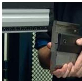
Adapters are used between the press brake's Clamping (or Tool Holder) and the top tool. Often they are used as an accessory to make the transition from one tool system to another. These adapters are supplied as modules in lengths of 150 and 515 mm. They are produced with extremely high precision, guaranteeing their interchangeability.
