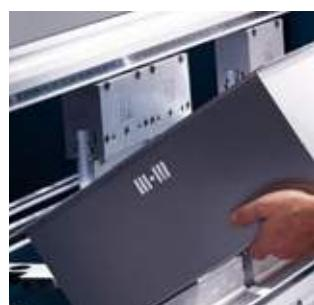
Extenders are used between the press brake's upper Clamping (or Tool Holder) and the top tool. Often they are used to heighten the top configuration, making it possible to bend deep boxes.
