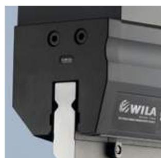
Guards are cover plates for the ends of the Tool Holders that make it easier to insert tools horizontally. In addition, Guards protect clamps and tools against damage.
