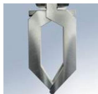
Because New Standard and American Style tools are symmetrical in relation to the centerline, these (top) tools can be easily rotated, such as when bending a reverse flange with a gooseneck tool.
