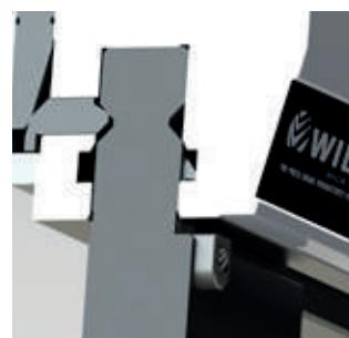
Tools are clamped using a pneumatically-controlled pair of self-adjusting wedges. When the wedges are engaged (clamped), they become an integral part of the tool. The Self-Locking® principle is suitable for clamping WILA's New Standard top and bottom tools (BLU and OZU). The Premium clamping is also released pneumatically.
