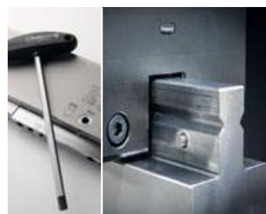
New Standard E2M® top and bottom tools are equipped with special (pre-assembled) bearings, which allow you to move the tools laterally in a non-clamped state quickly and safely.
