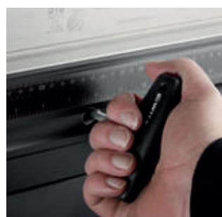
Ty-adjustment is crucial in determining the parallelism between top and bottom tools. Adjustment in Y direction makes it possible to fully compensate for unavoidable - cumulative - processing tolerances in the press brake. Either the top or bottom Tool Holder must be able to do this if one wants to achieve accurate and consistent bending results.
