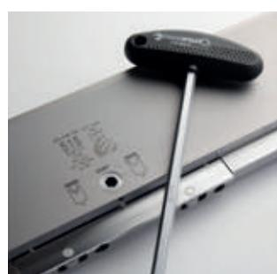
E2M® bottom tools are provided with an internal lift system. This system is applicable for a tool weight with a maximum of 140 kg and minimum tool length of 200 mm. Minimum width of the tool should be 30 mm.
