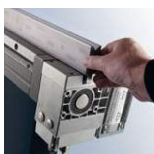
CRM7 is a CNC-driven drive motor which has been designed for New Standard Pro Crowning. This motor makes it possible to horizontally insert and remove bottom tools from both ends. The CRM7 motor is available for crowning lengths up to 4300 mm.
