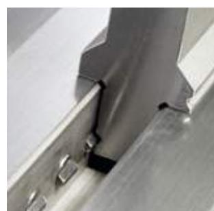
The V-Lock® improves the clamping and positioning of bottom tools. A groove in the tool tang allows specially designed clamping pins to automatically align and firmly clamp bottom tools in both X and Y directions.
