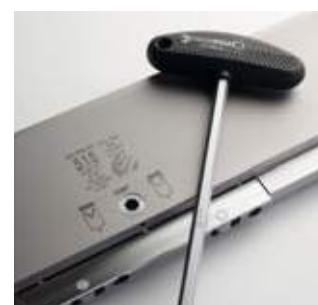
E2M® bottom tools are provided with an internal lift system. This system is applicable for a tool weight with a maximum of 140 kg and minimum tool length of 200 mm. Minimum width of the tool should be 30 mm.
