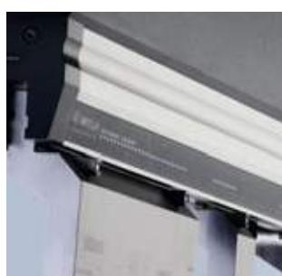
This intelligent ruler equipped with LED lighting immediately shows where tools must be placed in the Tool Holder. The Smart Tool Locator® also identifies the exact bending sequence.
