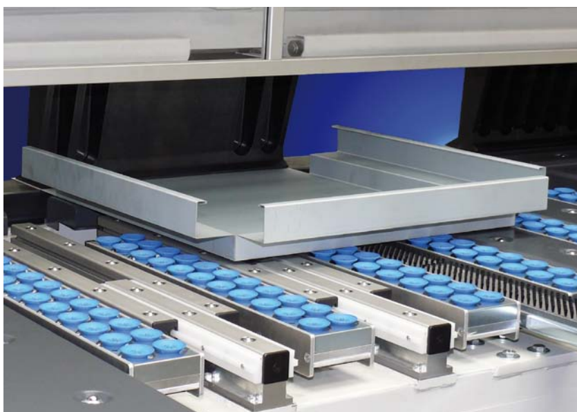
The PosLift gauging system positions the part for each bend
