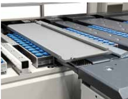
Accurate alignment of long and narrow parts with the active squaring arm.
