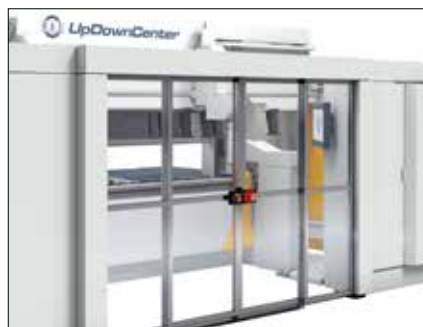
Machine with tool changer. Sliding glass doors preferably protect the folding beam area.
