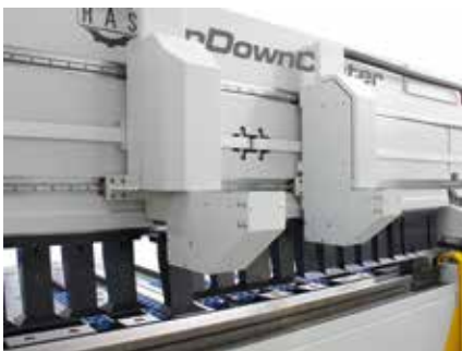
The automatic tool changer (78.33-2 & 78.43-2) sets up of even heavy tools.
