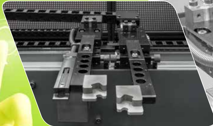
Backgauge with X-, R-, Z1+Z2- and Delta X-axes
