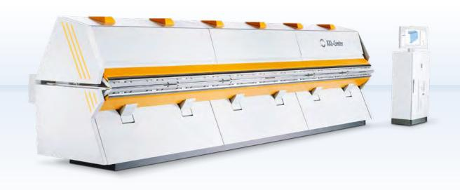
The XXL long folding center automatically inserts, squares, positions to the bend line, and folds the flanges up or down. No more rotation. No more complicated handling. No more second or third operator. The XXL-Center automatically produces precision long parts in record time.
