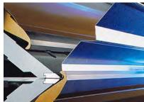
No part rotation required since the machine bends up and down. High productivity due to fast bending cycles.
