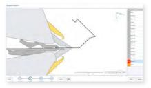
2D or 3D simulation of the bending sequences and visualization of possible collisions.
