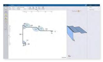
Drawing of a profile on the touchscreen monitor. Automatic programming of the bending sequence with just one mouse click. No expert knowledge required. New parts can be tested for feasibility in the office using the Office programming software.
