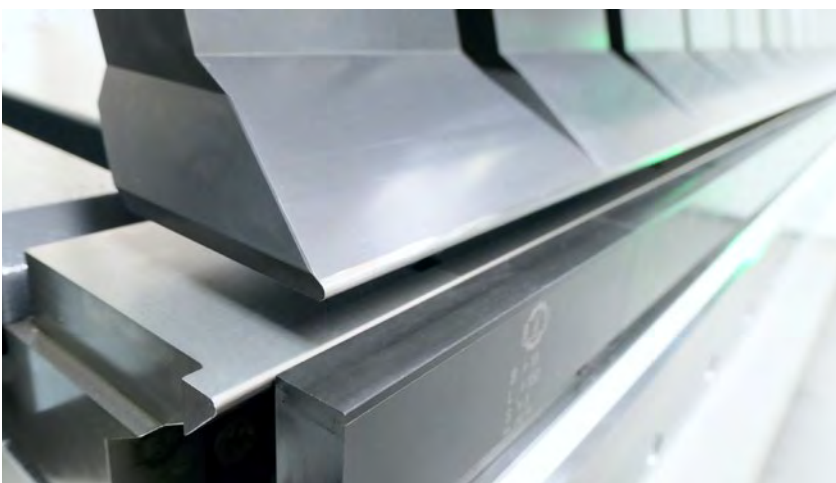
Some materials require the use of radius tools in the upper and lower beams. Combined with folding beam tools with plastic inserts, perfect surfaces will be created.
