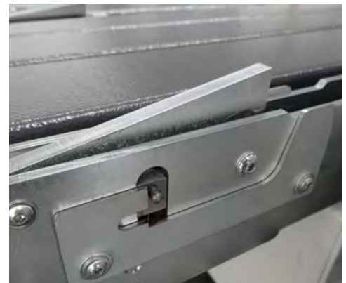
If the outside edges of the blank are not straight, individual stop fingers can be deactivated.
