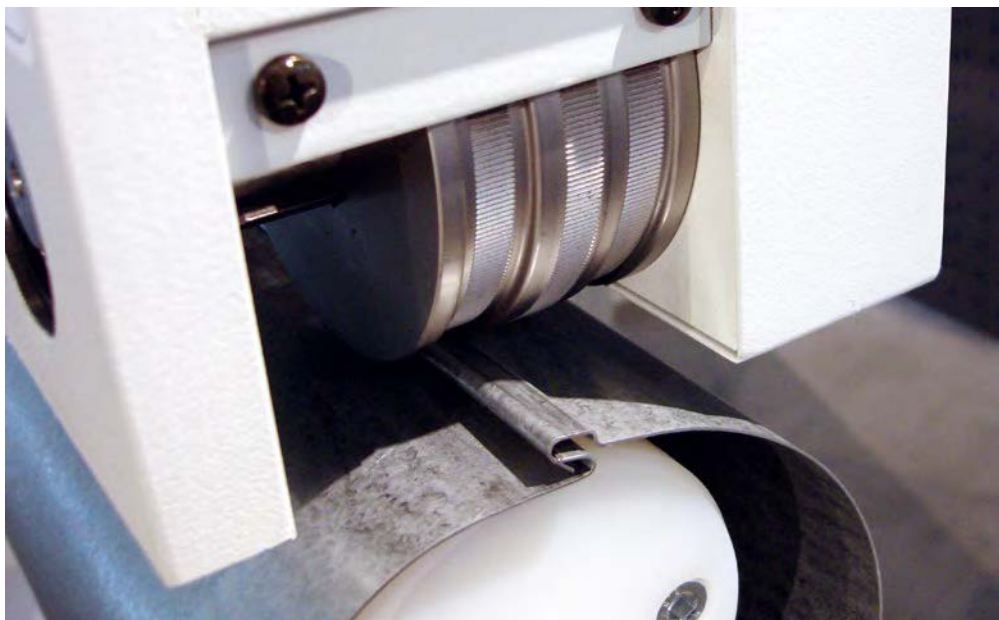
Closing of longitudinal seam (tube seam) on round tubes
