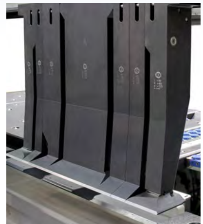
Upper beam tools as tall as 600 mm
