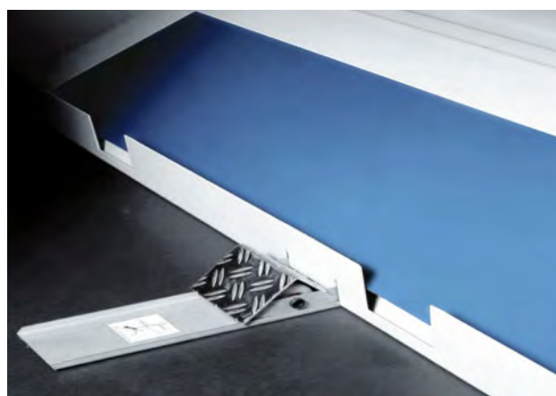
The foot lever switches the parts chute direction.
