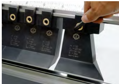
Tools with quick clamping system
