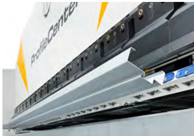
Complex part geometries can be bent due to the large free space around the tools.
