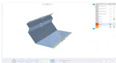
Automatic programming of the bending sequence in the graphics software.
