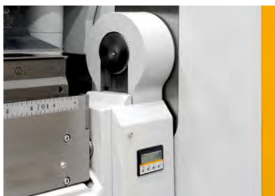
Optional digital display for folding beam adjustment.
