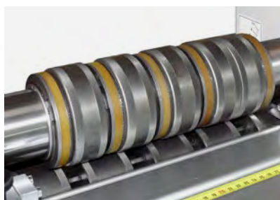
Rolls for standing seam and snap-lock seam.
