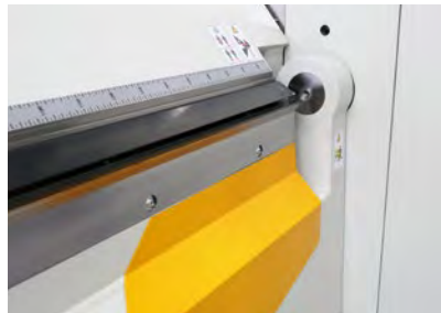
Alternative: XL folding beam with extra free space.
