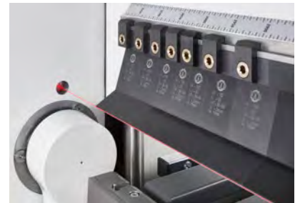
A laser automatically recognizes the exact tool height.
