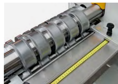
Tape measure for quick roll positioning.
