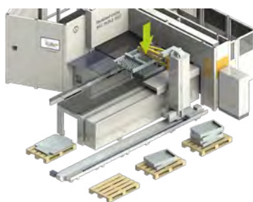
Picking up the bent part by the suction frame of the palletizer
