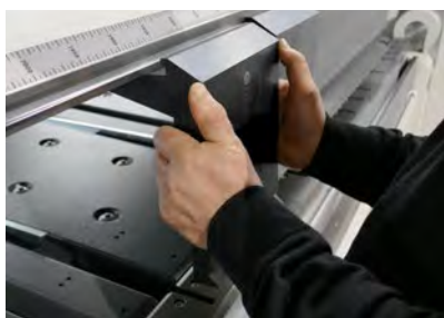
Quick tool set-ups due to the automatic tool clamping system.
