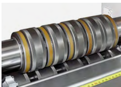
Rolls for standing seam and snap-lock seam.
