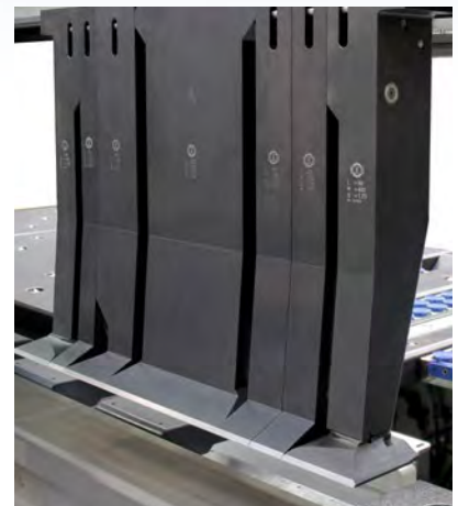
Upper beam tools as tall as 600 mm
