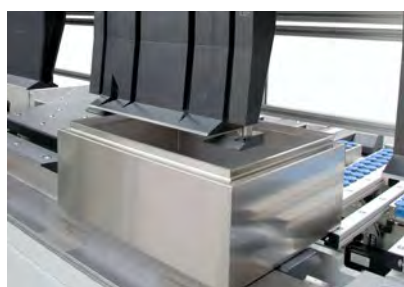
Upper beam tools for boxes up to 600 mm tall.
