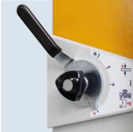
Blade clearance adjustment on RAS PRIMEcut.
