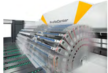
Automatic bending with fast cycle times. The workpiece does not have to be positioned at the stops during bending process.
