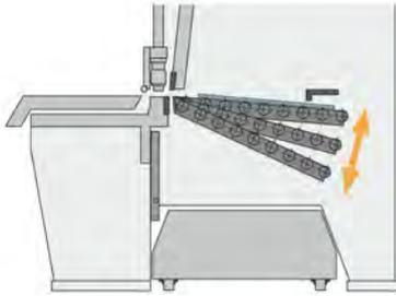
After the cut, the sheet support system can move into four different part delivery positions. Down quietly and gently.
