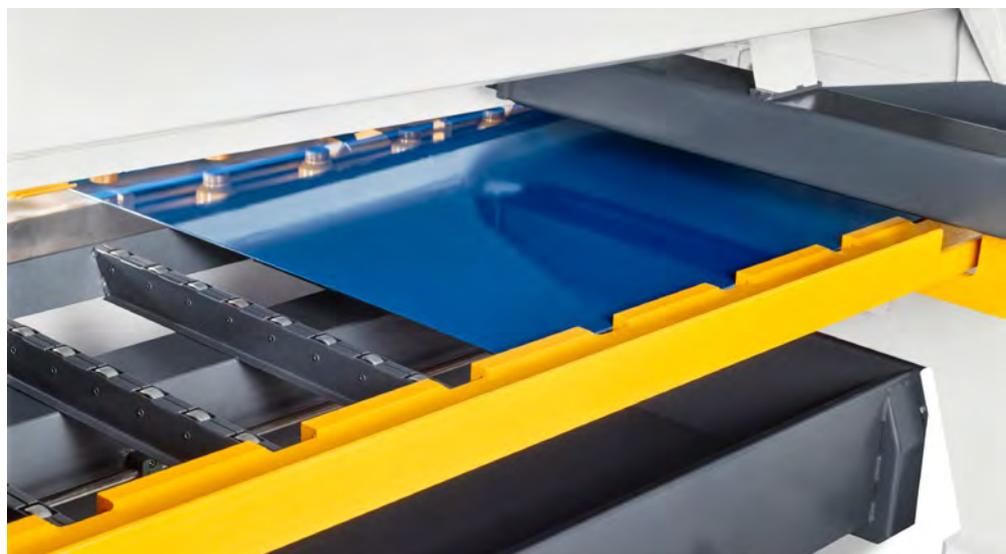
The sheet support system guides even thin materials exactly to the CNC backstop.
