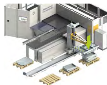
Horizontal stacking of a bent part on a pallet
