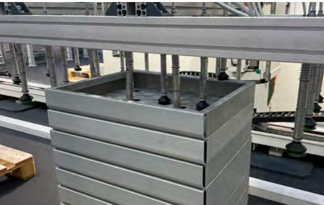
Loading system for automatic feeding of blanks from a stack of sheets with sorted and edge-precisely stacked sheets
