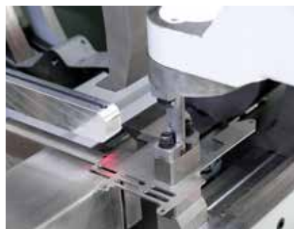
Measuring the parts by a laser scanner.
