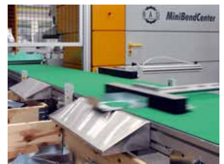
Unloading of finished parts into bulk material containers.
