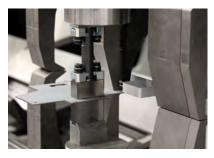
Several bending stations can be set up along the bending line. Complex bent parts are thus completed in one pass.
