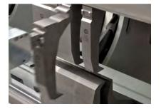
The automatic tool change allows quick part change and bending of small batches.
