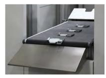
Bent parts that cannot be stacked can be discharged via the outfeed conveyor.
