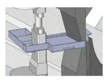
Simple Office programming starting from a STEP file of the bent part with 3D visualization of the bending sequences.
