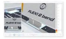
The 3D simulation shows the automatically programmed bending sequence.
