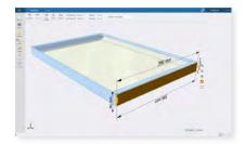
Part geometries can be added by drawing, table input, or STEP/dxf import.
