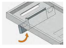
The DownTools can be used to bend louvers, multi-sided parts, and flanges bent inward without an additional tool set-up.
