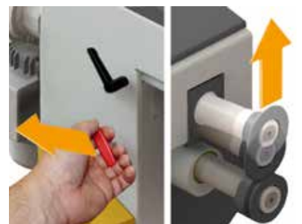
UnLock function opens the wheels immediately in an emergency.
