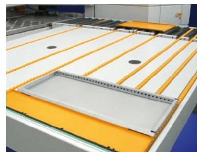
The runout extension moves the finished part to the multiple finished part buffer.
