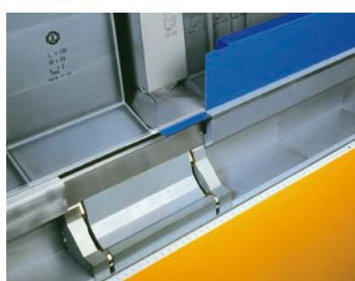
UpDown-tool inactive position (collapsed)
