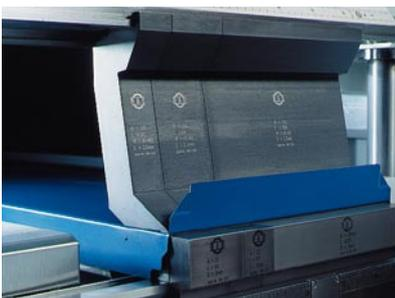
Segmented lower beam tooling for reverse flanges of up to 40 mm (1.575")
