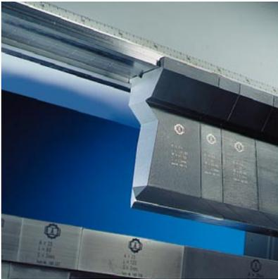
Automatic upper beam tool clamping system
