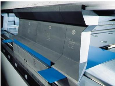
Segmented folding beam tools for flexibility in any situation
