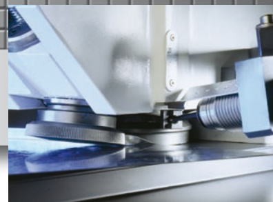
Automatic material guiding for flange heights of 8 or 10 mm (5/16" or 3/8") (Option)
