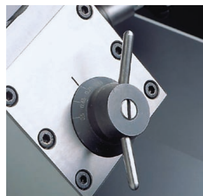
Variable material thickness adjustment from 0.5 to 1.5 mm (26 to 16 Ga.)
