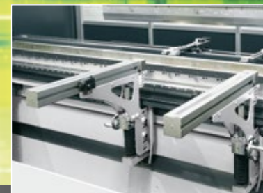
Moveable support arms adjustable in height
