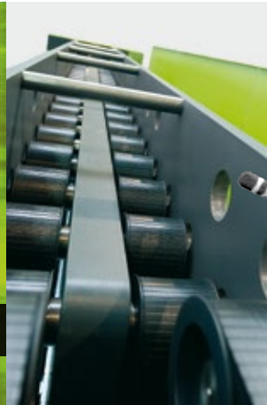
Roller drive with 4 servo motors
