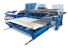
The loader is located on the right side of the punching machine. The loader replaces the front table and is constructed with the extension tables as a complete unit.
