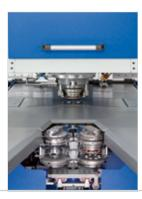
1 head with 8 stations tool changer 28to 40 mm stroke Max. 76mm outside diameter Up to max. 64 tools (Revotool)
