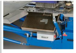
Small parts chute 100x120mm und 670x670mm
